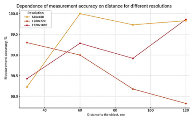
Fig. 5. Evaluation of resolution impact on distance measurement accuracy
