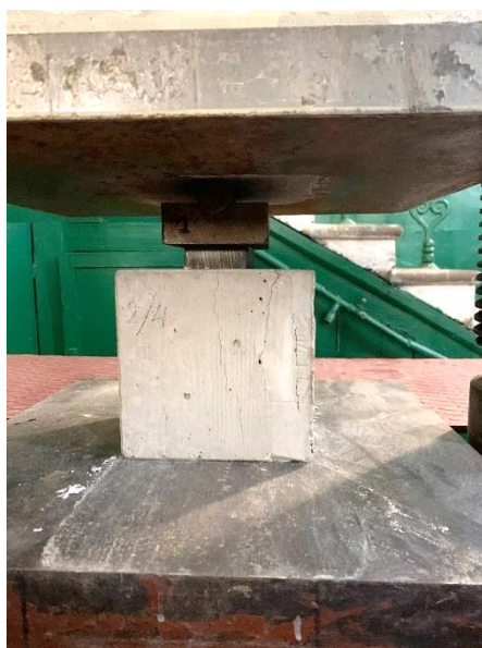
Figure 2 – Sample testing for local compression in the press III-125
