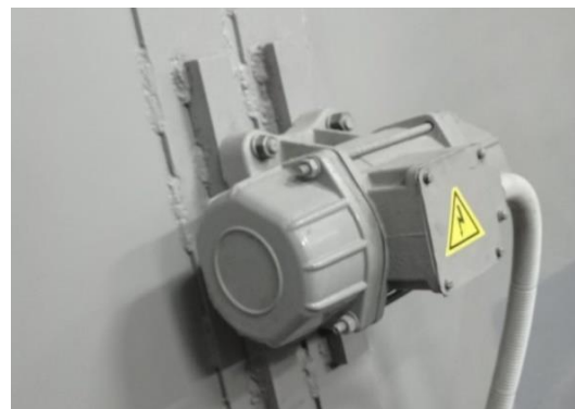
Figure 11 – Vibrator is installed on the hopper
