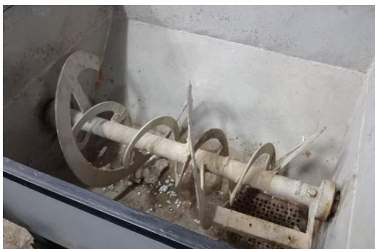
Figure 10 – Mixer for preparing construction mix
