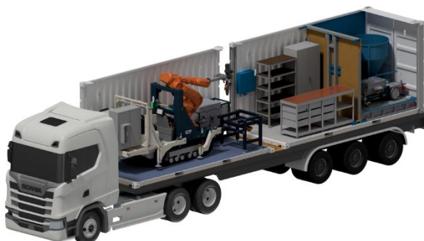
Figure 4 – Transportation of the mobile 3D Printing system
