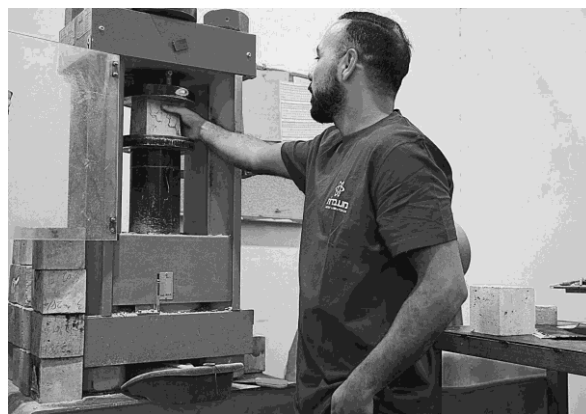
Figure 2 - The method for testing the compressive strength of concrete.
