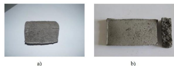
Figure 5 - Illustration of the items fragments formed: a) - in the form of plates; b) - in the form of films
