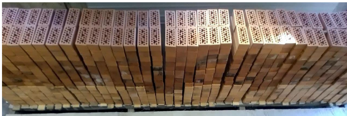
Figure 1 – General view of specimen 1.7–2.3–1.7 SCCS 0.53 × 6.0 under maximum loading.
